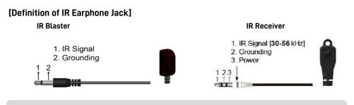
You can buy any IR extension cables in the market that are compatible to the definition of the IR sockets for the extender if necessary for replacement use. However, IR cables longer than 2m (6-ft) may not work.
